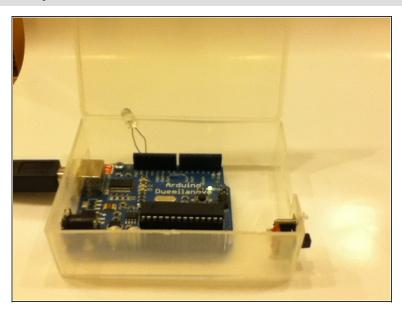
Now just connect the LED between pin 13 (+) and GND (-), and plug the Arduino into your computer.
